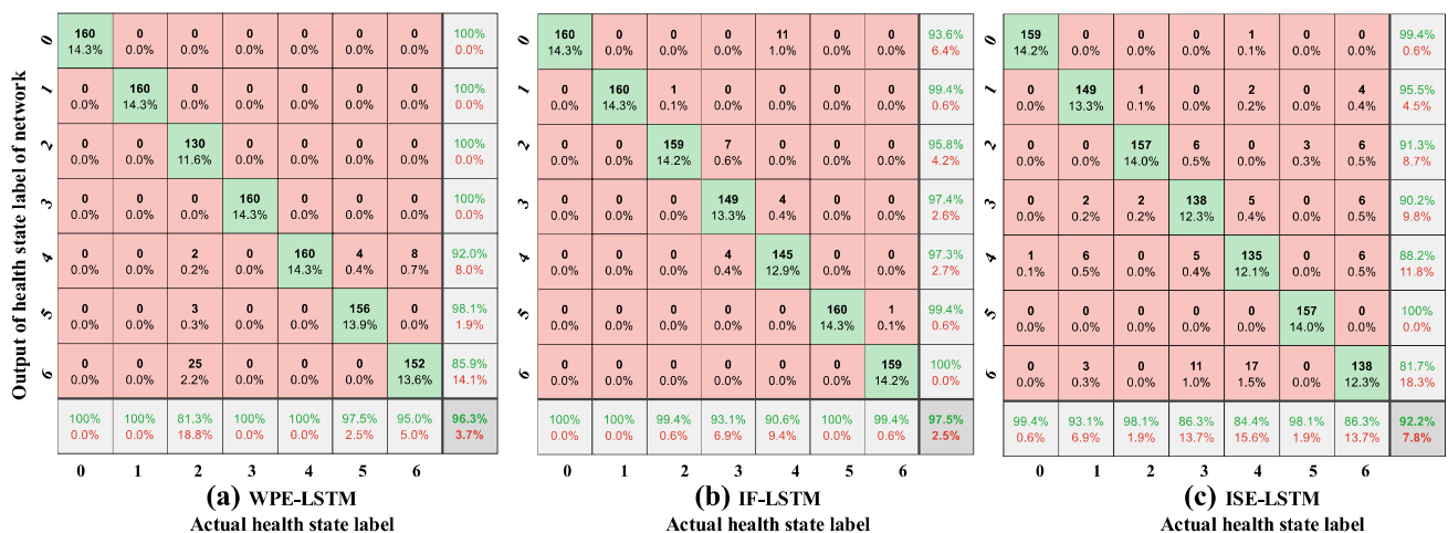
Fig. 22 Confusion matrix of case study 3 under motor speed 1500, given by the traditional method
