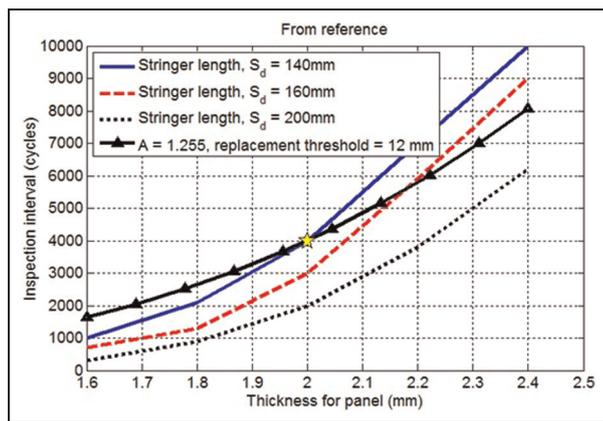
**Figure 7.** Comparing the sensitivity of inspection interval for an optimal set of parameters and reality.
