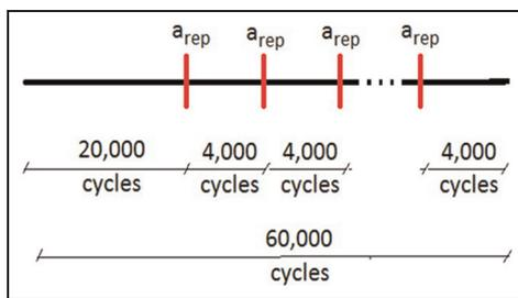
**Figure 2.** Schedule of the scheduled maintenance process. Cycles represent the number of flights.
