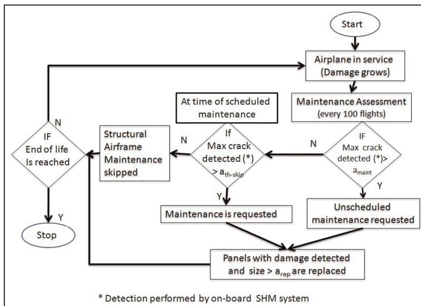
Figure 4. Flowchart depicting maintenance scheduling and assessment procedure for CBM-skip.
