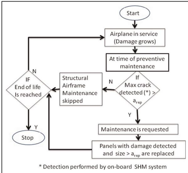
Figure 3. Flowchart of Sched-SHM maintenance process.
