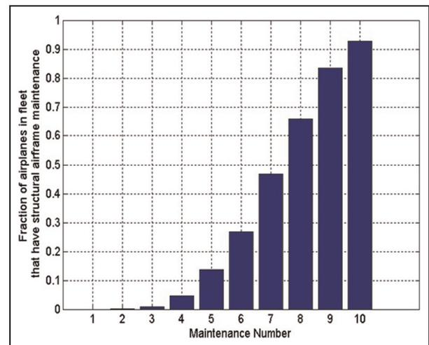
**Figure 5.** Fraction of airplanes undergoing structural airframe maintenance at each scheduled maintenance.
