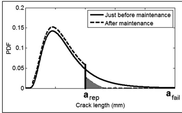
**Figure 1.** The effect of inspection and replacement processes on crack length distributions. PDF: Probability density function.
