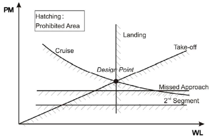
Figure 5. Example of matching chart for preliminary aircraft sizing, typical of a propeller airplane.
